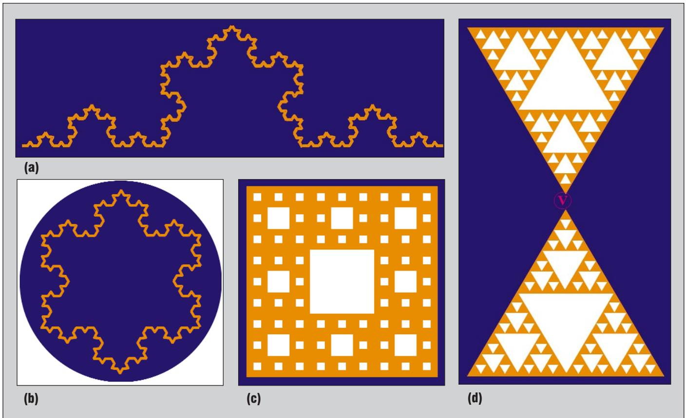
▲ **Figure 3. Various fractal antenna elements: (a) Koch dipole, (b) Koch loop, (c) Sierpinski dipole, (d) Cantor slot patch**
