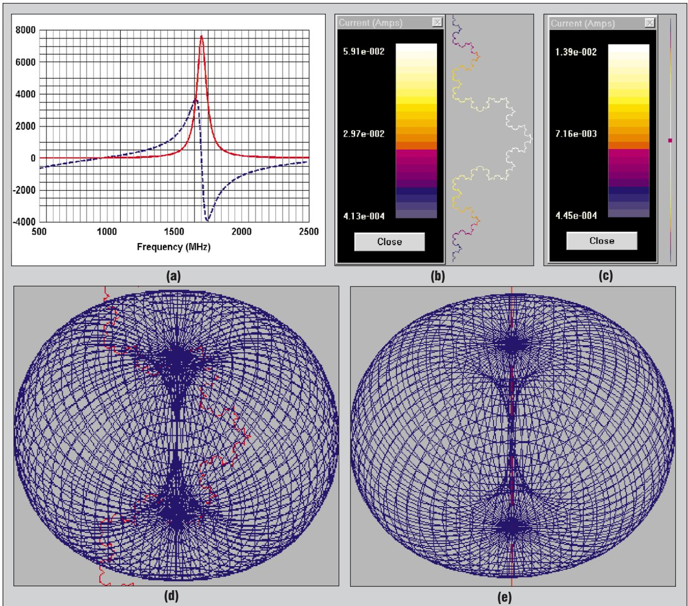
▲ **Figure 4. Koch dipole and regular dipole: (a) Input impedance of a Koch dipole; (b) Current distribution of the Koch dipole at 961 MHz; (c) Current distribution of the regular dipole at 1.851 GHz; (d) 3-D radiation pattern of the Koch dipole at 961 MHz; (e) 3-D radiation pattern of the regular dipole at 1.851 GHz. (continued on next page)**
