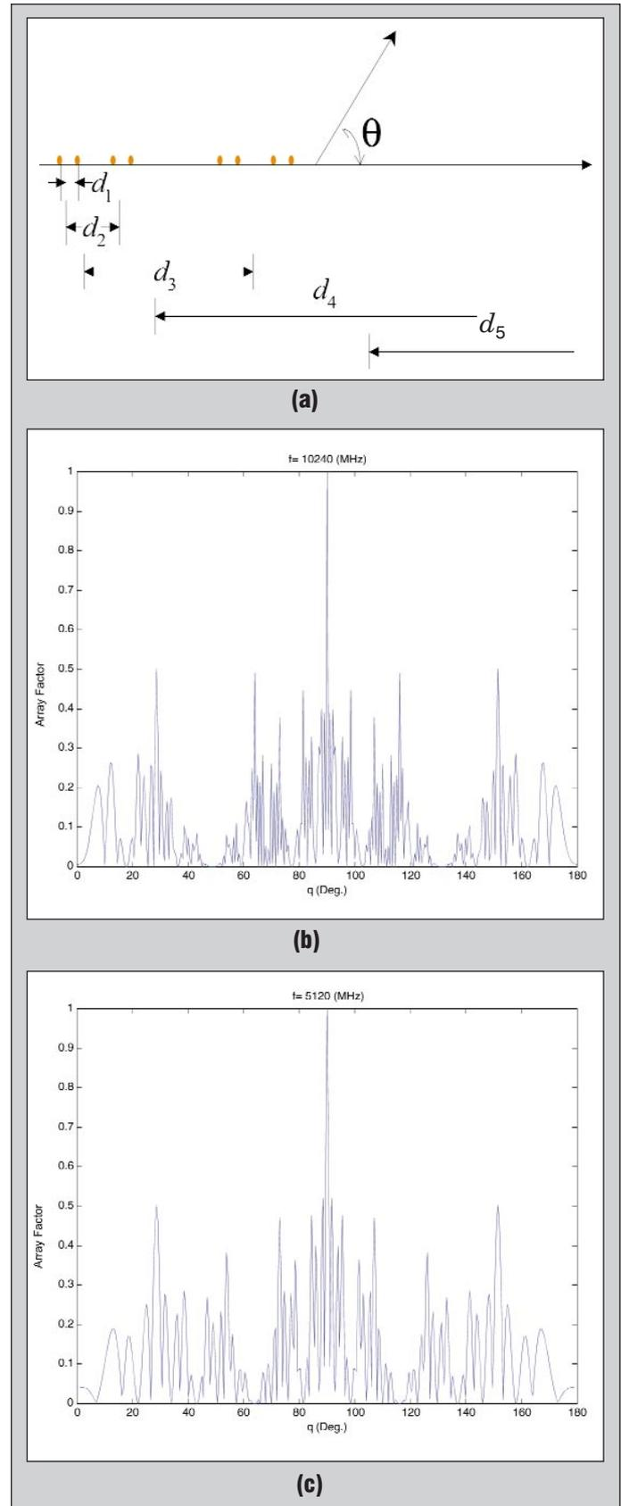
▲ Figure 6. Array factor of a linear Cantor array: (a) Cantor linear array; (b) Array factor at  $f = 10240$  MHz; (c) Array factor at  $f = 5120$  MHz. (continued on next page)
