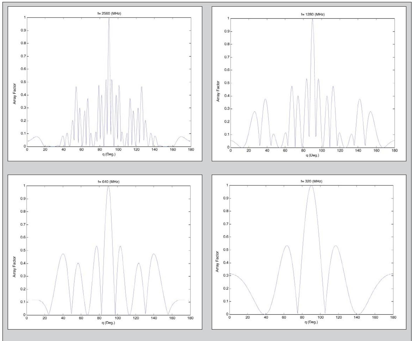
▲ **Figure 6 (continued).** Array factor of a linear Cantor array: (d) Array factor at  $f = 2560$  MHz; (e) Array factor at  $f = 1280$  MHz; (f) Array factor at  $f = 640$  MHz; (g) Array factor at  $f = 320$  MHz.
