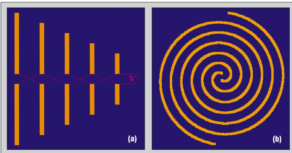
▲ Figure 2. Frequency independent antennas as fractal antennas: (a) Log-periodic dipole antenna, (b) Spiral antenna
