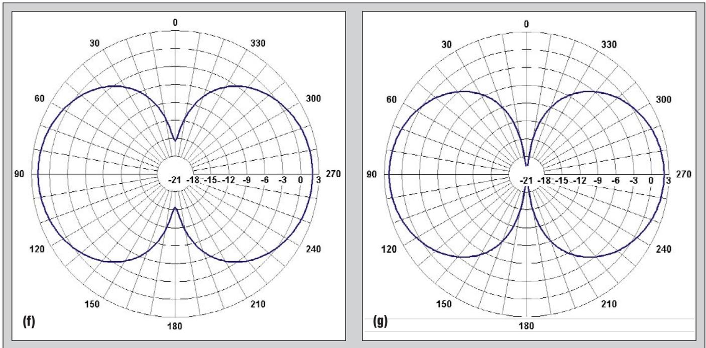
▲ **Figure 4 (continued).** Koch dipole and regular dipole: (f) Radiation pattern of the Koch dipole at 961 MHz; (g) 3-D radiation pattern of the regular dipole at 1.851 GHz.
