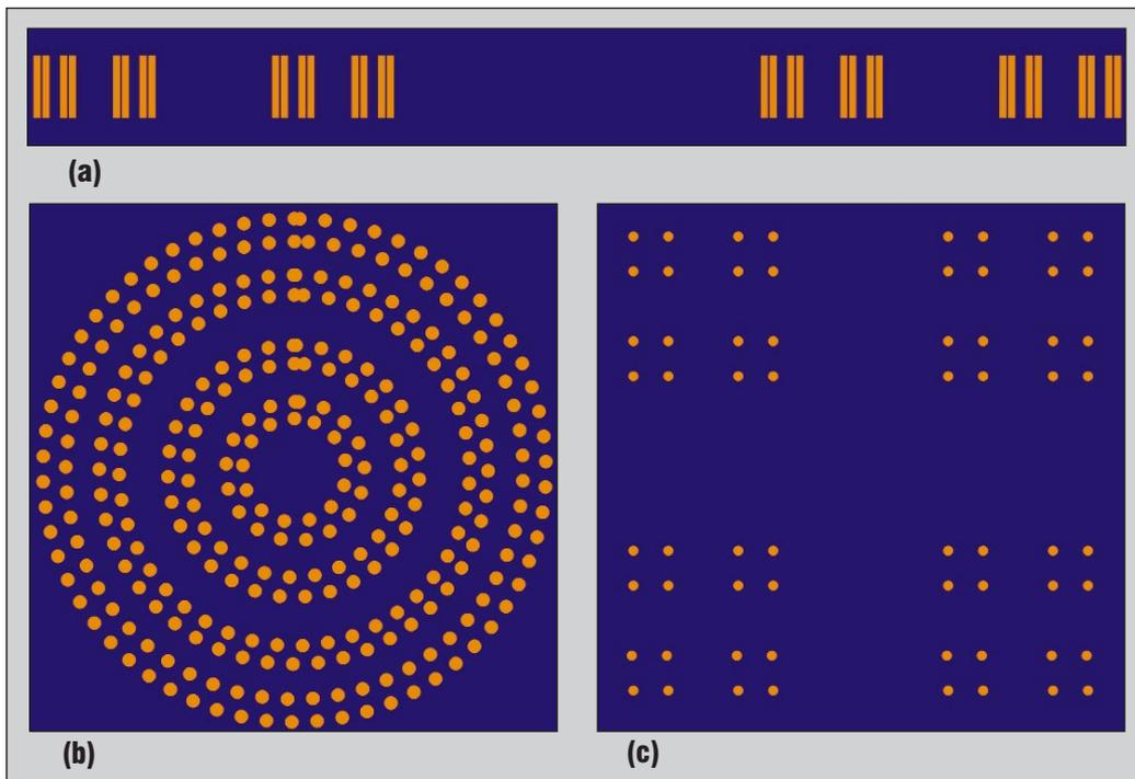
▲ **Figure 5.** Various fractal antenna arrays: (a) Cantor linear array; (b) Cantor ring array; (c) Sierpinski carpet planar array.
